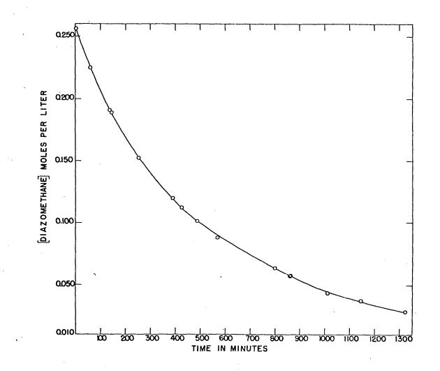
Figure 2. Reaction of diazomethane and 2,4-pentanedione in 1,2-dimethoxyethanebenzene at 27.0°. Concentration of 2,4-pentanedione as a function of time. Experimental values are represented by 0. Corrected values used in calculation of rate constants are represented by x.
