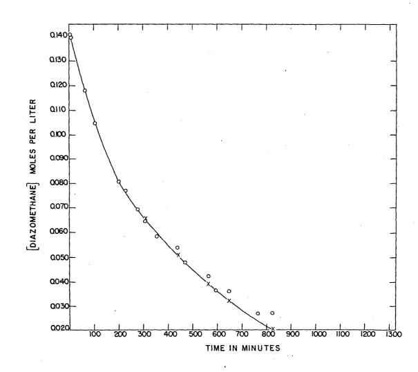
Figure 4. Reaction of diazomethane, 2,4-pentanedione, and p-toluenesulfonic acid in 1,2-dimethoxyethane-benzene. 2,4-Pentanedione as a function of time. Experimental values are represented by 0. Corrected values used in calculation of rate constants are represented by x.
