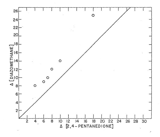
Figure 6. Reaction of diazomethane and 2,4-pentanedione in 1,2-dimethoxyethane-benzene at 27.0°. Change in diazomethane concentration versus change in 2,4-pentanedione concentration. See page 41.
